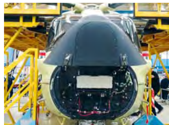
Leonardo's new Osprey airborne surveillance radar uses flat panel antennae to dispense with the necessity of mounting a radome beneath the aircraft, and will equip the AW-101 helicopters of the Royal Norwegian Air Force.
