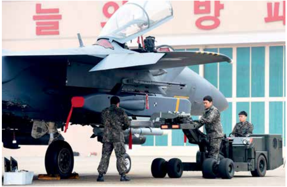
A RoKAF's Boeing F-15K Slam Eagle strike fighter being fitted with a Taurus KEPD-350E.
