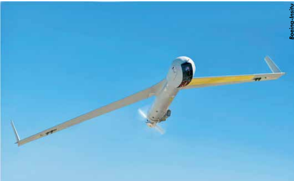
Small UAVs such as the ScanEagle can cover large swathes of land with specialised payloads.
