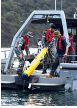
Australian Mine Warfare Team 16, recover a General Dynamics Bluefin 9 AUV from a Mine Countermeasure Support Boat (MCMSB) in January-February 2020. (Australian Department of Defence).
