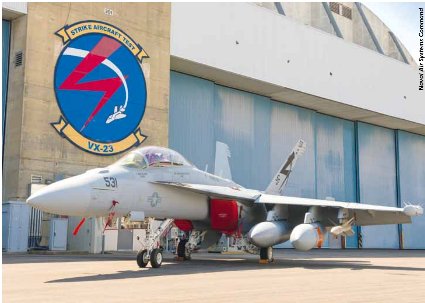
An EA-18G Growler assigned to Air Test and Evaluation Squadron 23 loaded with a ALQ-249 Next Gen Jammer pod on station 3 (middle).
