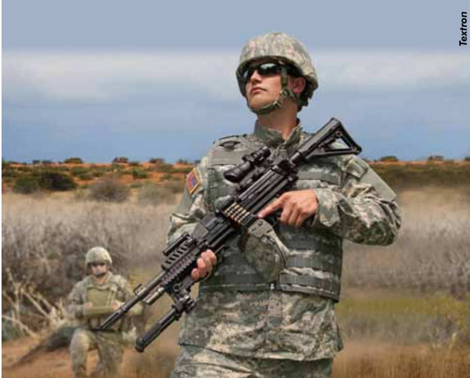
The US Army is evaluating three candidates for its Next Generation Squad Weapon. One of them being offered by Textron uses a unique CT Cased Telescoped ammunition that is lighter and shorter than conventional cartridges. The LMG version (shown) uses belted ammunition with polymer links.
