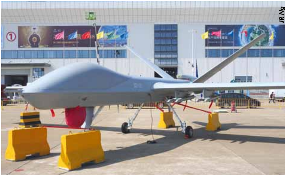
A PLAAF Wing Loong-2 MALE UAV, otherwise known as the Gongji-2 (GJ-2).
