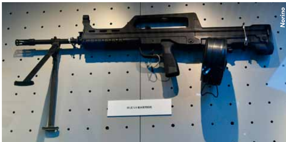
The Peoples Liberation Army (PLA) has fielded its QBZ-95 family of squad weapons which includes the QBB-95 Light Support Weapon. The latter is designed with a heavy barrel for sustained automatic fires. It uses an 80-round drum magazine but also accepts the standard 30-round box magazine. The latest model QBB-95-1 fires a heavier 5.8×42mm DBP10 round that offers improved performance at range.
