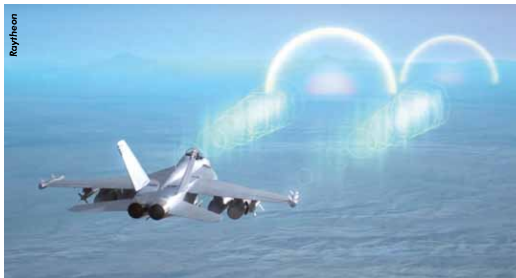
An interesting perspective of electronic attack activity radiated from two ALQ-249 NGJ mid-band pods.
