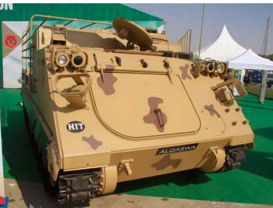
▲ The Al-Qaswa is an armoured personnel carrier (APC) designed and manufactured in Pakistan by Heavy Industries Taxila (HIT). It is a modernised version of the M113-A2-Mk1 APC. Operating as a logistical vehicle, it can carry six tonnes of military supplies and is adaptable to fulfil a number of formats.
