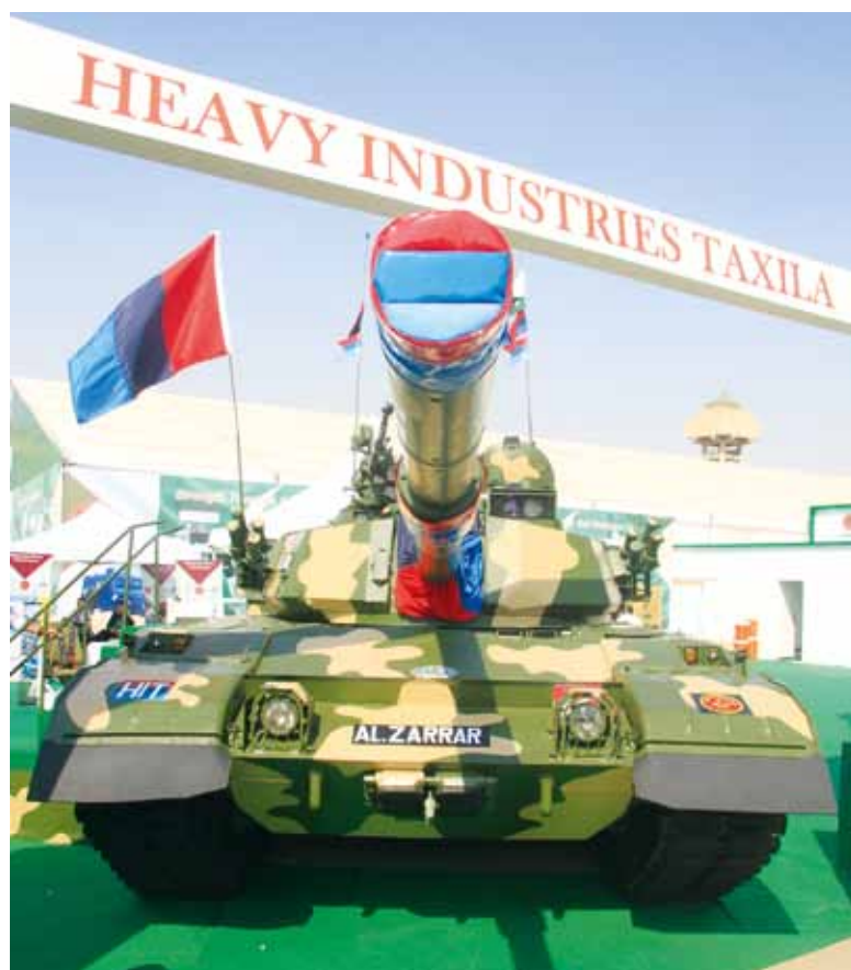
▲ The Al-Zarrar is a second generation main battle tank (MBT), which has been in service with the Pakistan Army since 2004. The tank is named as Al-Zarrar, which means 'main striker' in Arabic and Persian languages. It has a 125 mm smoothbore gun as primary weapon, weighs 44 tons, has a crew of four and can reach 65km/h.
