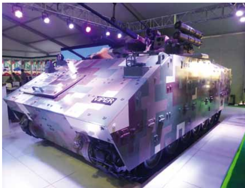
◀ The Multi-Purpose Infantry Fighting Vehicle (MIFV) Viper from Heavy Industries Taxila has Stanag Level IV all round vehicle protection. It has an unmanned remotely controlled turret with a crew capacity of 13, a maximum road speed of 75km/h and a cruise range of 500km. This version was displayed in Hall 8 at IDEAS on the company's stand.
