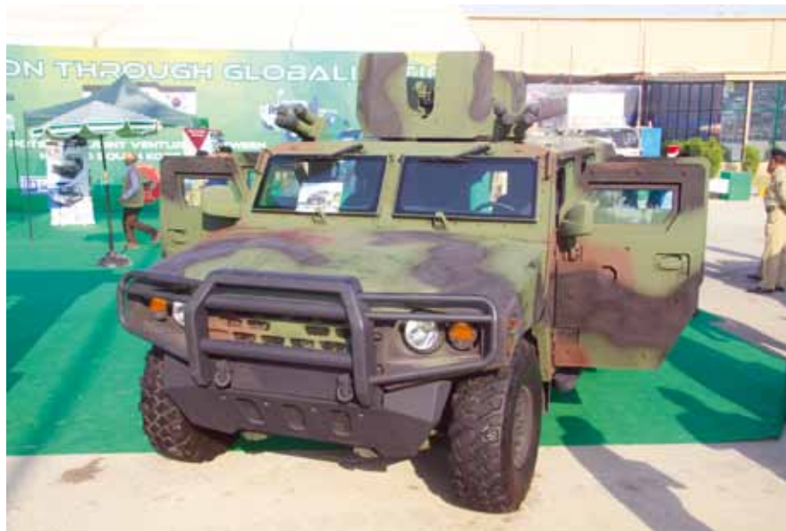
◀ The Multi-Purpose Infantry Fighting Vehicle (MIFV) Viper from Heavy Industries Taxila has Stanag Level IV all round vehicle protection. It has an unmanned remotely controlled turret with a crew capacity of 13, a maximum road speed of 75km/h and a cruise range of 500km. This version was displayed in Hall 8 at IDEAS on the company's stand.
