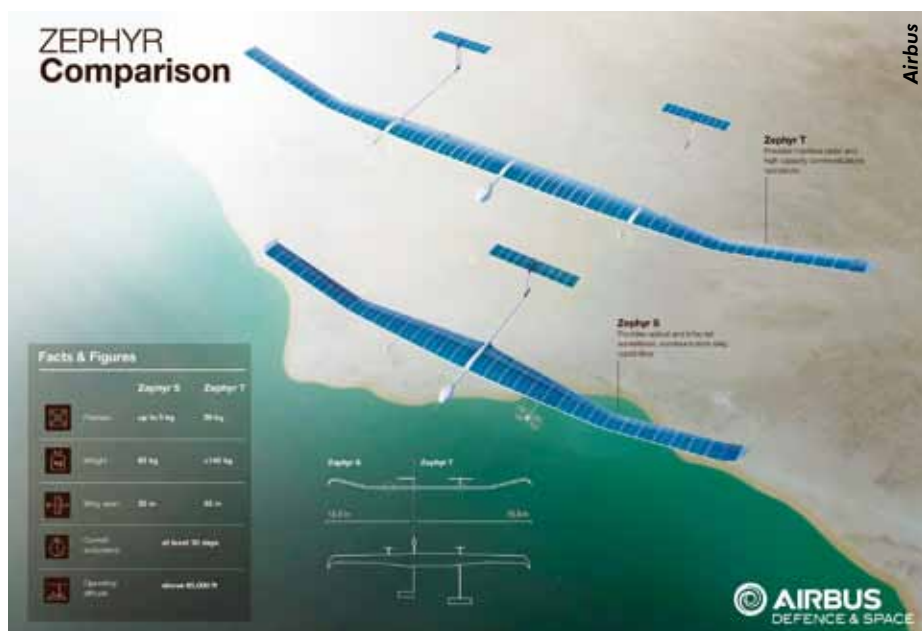
The Zephyr-S/T will be available in two variants that will have different payloads, both of which are solar-powered and can stay aloft for days on end.
