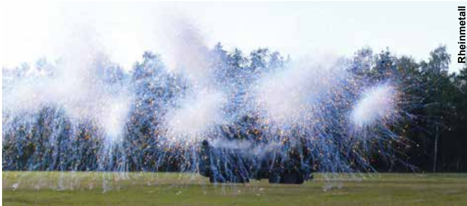
Vehicle-launched rapid screening systems like Rheinmetall's ROSY offer an immediate response to contact by obscuring the vehicle and disrupting weapon guidance systems.
