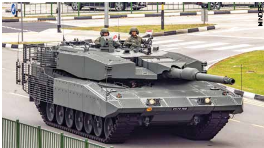
The level of protection improvement possible is evident in Singapore's Leopard 2SG tank that incorporates AMAP protection and survivability upgrades.
