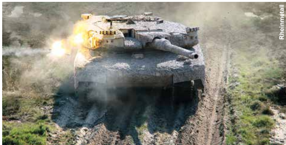
Rheinmetall's Strike Shield, shown here on a Leopard 2 MBT, defeats an incoming projectile in live-fire tests. Its first operational fielding will be on Hungary's Lynx IFVs.
