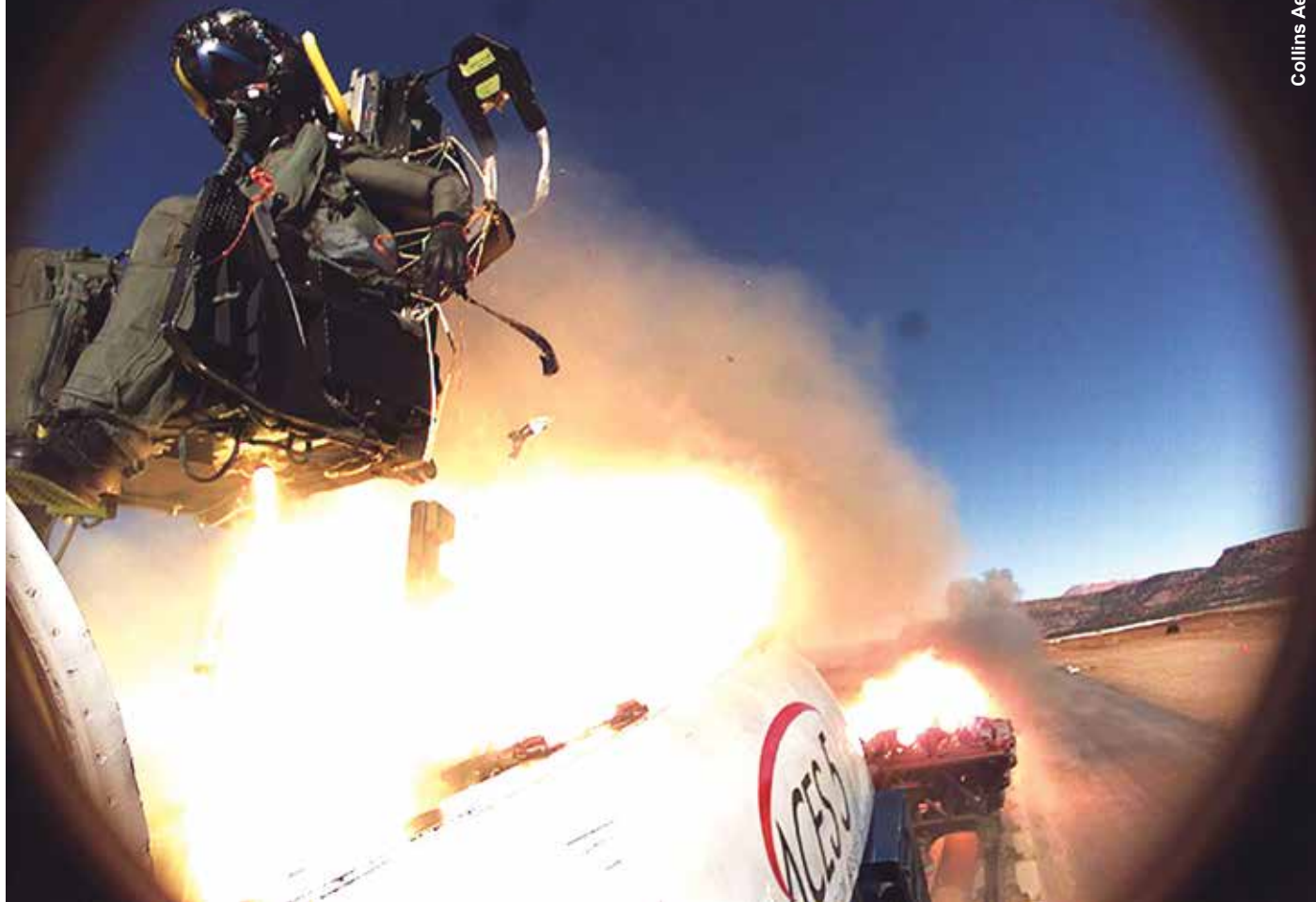
A test firing of the Collins Aerospace ACES 5 ejection seat using a crash seat dummy.
