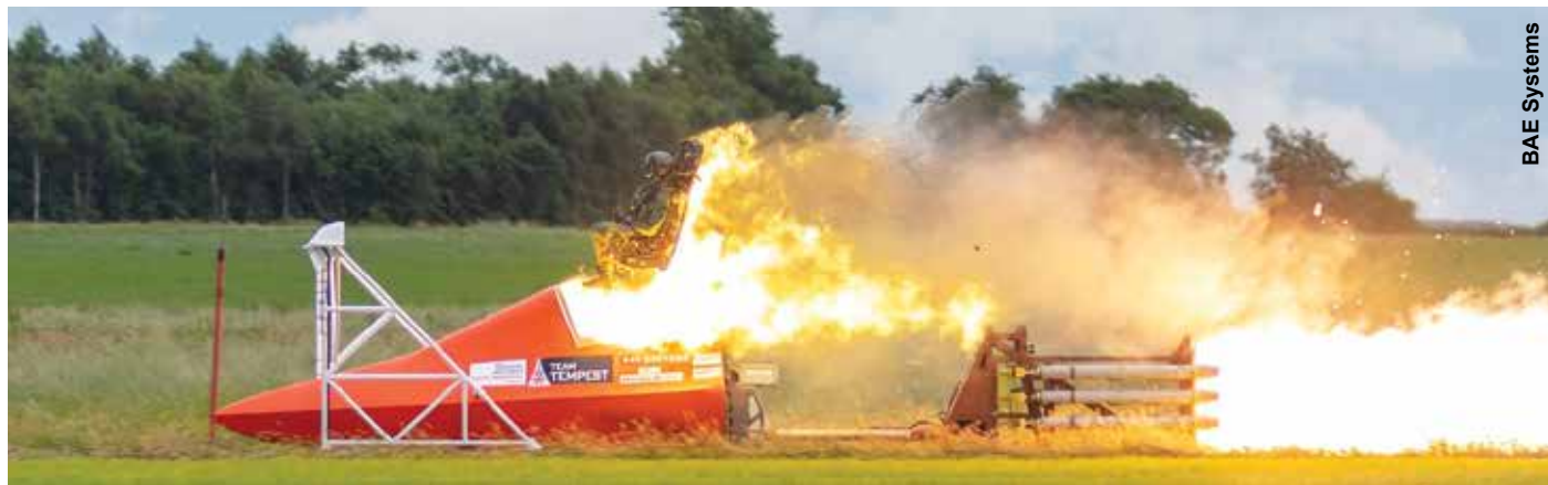
BAE Systems are using a rocket-propelled sled to test future ejection seat systems for the next generation Tempest fighter.
