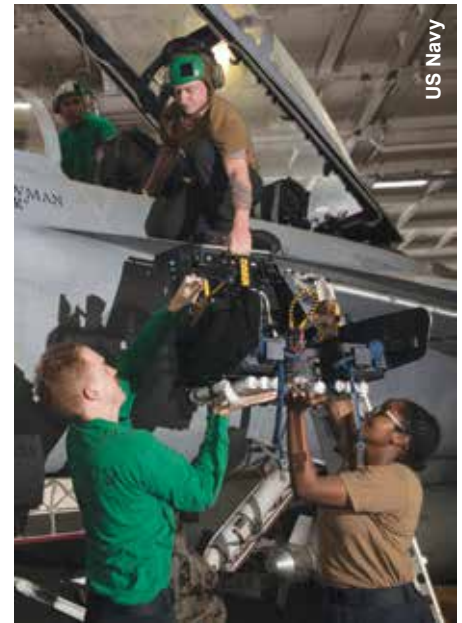
The Martin-Baker Navy Aircrew Common Ejection Seat (NACES) being removed from a US Navy F/A-18E Super Hornet.
