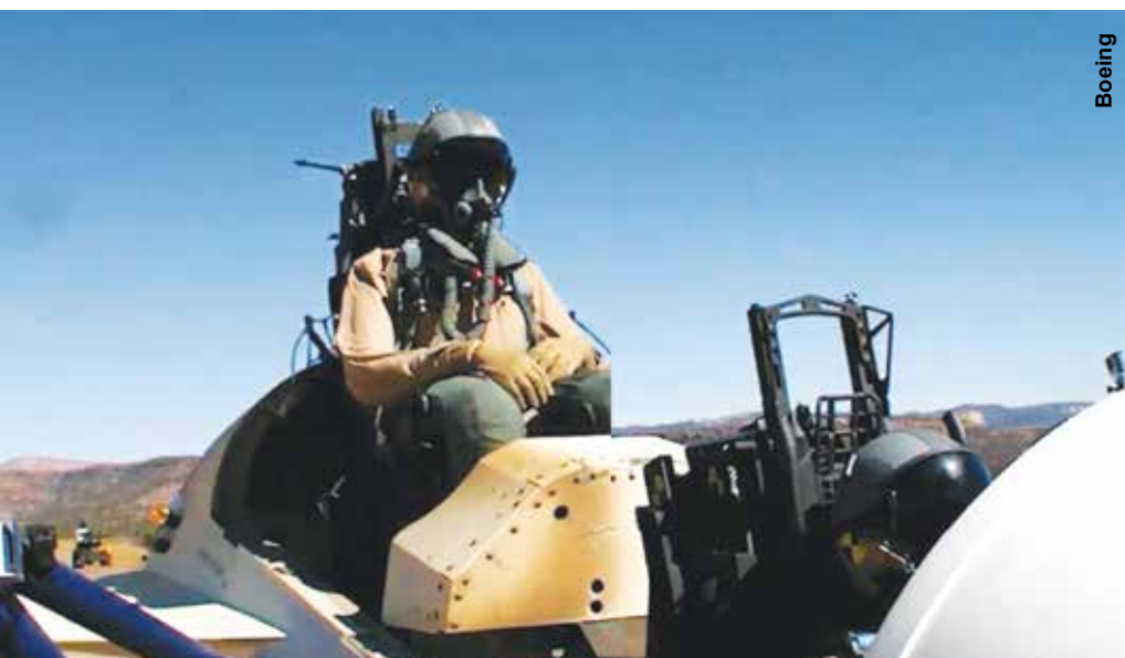
A crash seat dummy used for a test of the next generation ejection seat (NGES) for the Boeing T-7A Red Hawk trainer.
