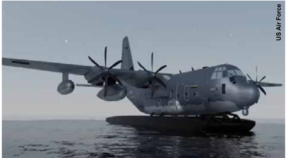
At the Air Force Association 2021 Air, Space and Cyber Conference, AFSOC announced the development of the MC-130J Combat Talon II Amphibious Capability. The removable amphibious float modification allows runway independent landing.
