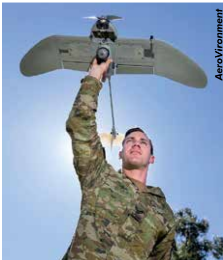
Looking for all the world like a model aeroplane, the 1.02m wingspan AeroVironment Wasp UAV is hand-launched, is equipped with a Mantis i22 EO/IR payload and has a range of over three miles (5km). Overall UAVs (as opposed to commercially available hobby drones) can range in size and capability from nano-drones through Wasp-sized vehicles to multi-sensor platforms such as the Global Hawk which has a wingspan that is similar to that of a Boeing 737 airliner
