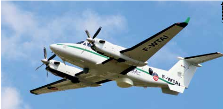
Textron Aviation's King Air 350 business aircraft is one of the world's most popular airframes for conversion into specialised airborne ISR platforms. Shown here is a King Air 350ER ISR aircraft that was produced by Swiss contractor Corporate Aircraft for an un-named North African customer. As such, F-WTAI has been fitted with an X-band Gabbiano T200 surveillance radar, an EO imager, an AIS application and Leonardo ATOS control system application
