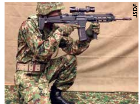
Japan's Defense Agency in August 2020 selected the Type 20 from Howa for fielding to its Self Defense Forces. Type 20's design incorporates many of the features that are becoming standard in current weapons such as ambidextrous controls, the Picatinny rail, and optical sights.
