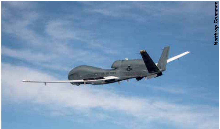
The Battlefield Airborne Communications Node (BACN) system is hosted on high-altitude aircraft such as the Global Hawk to provide persistent connectivity and operational support as part of the BACN programme.
